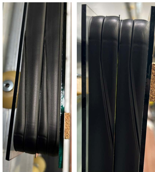
Figure 5. The TPS splice, where the spacer loop closes, is a core feature, maintaining a seamless, airtight connection that preserves the continuous bond.
