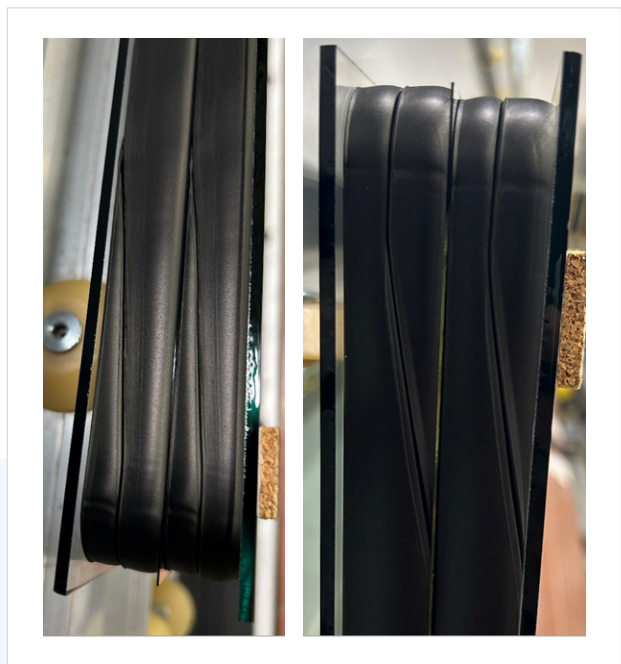
Figure 5. The TPS splice, where the spacer loop closes, is a core feature, maintaining a seamless, airtight connection that preserves the continuous bond.
